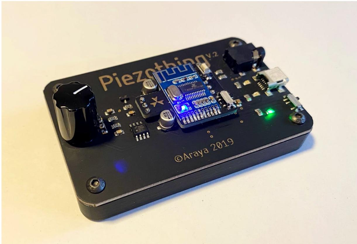
The BT is a Piezothing with an added Bluetooth transmitter board that allows you to stream the audio from the unit to a portable speaker, audio receiver or computer.
