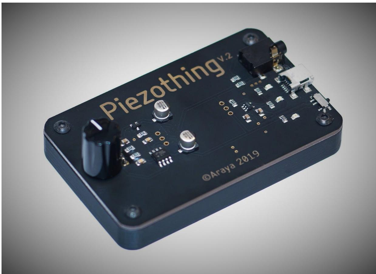
The **Piezothings** is a small feedback instrument containing a piezo microphone, a FET preamp, an amplifier and a small high quality transducer. The mechanical feedback through an object touching the mic and transducer produces both a physical signal vibrating the surface it is placed on as well as an electronic signal available at the headphone/line output.
